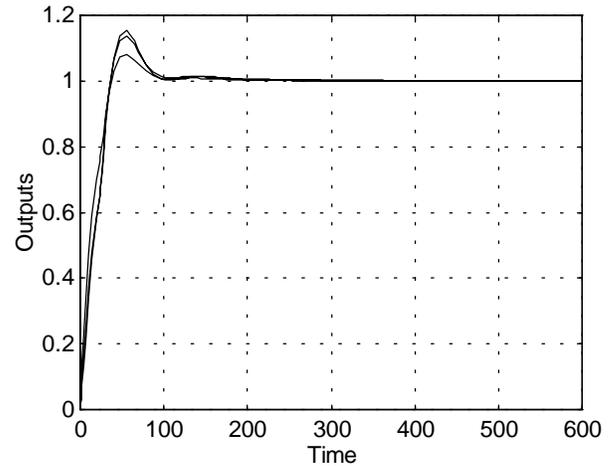
Figure 14. The pre-compensated closed loop system step response with PID controller.
