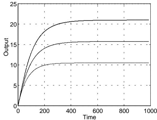
Figure 3. The open loop step response (Zone 2).
