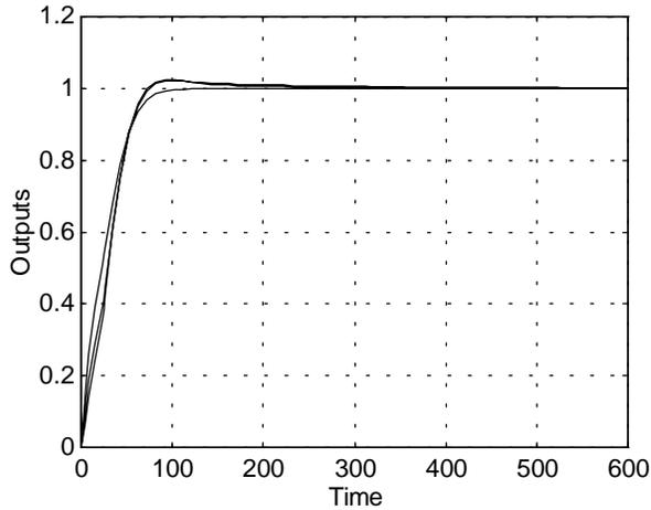
Figure 13. The pre-compensated closed loop system step response with PI controller.
