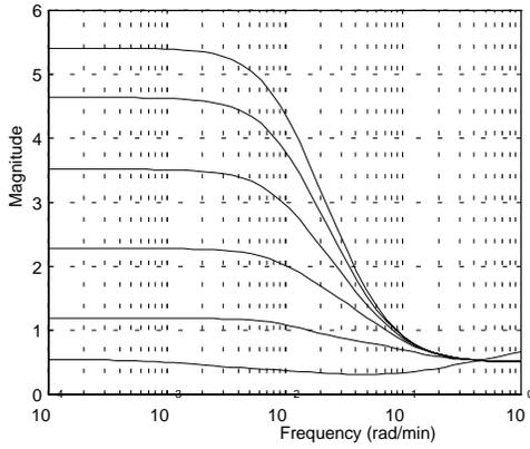
Figure 7. The principal gains of the open-loop system (controller + plant).
