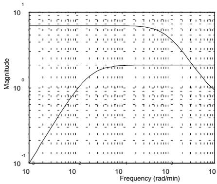
Figure 5. The nominal performance ( $1/w_p$ ) and robust stability ( $1/w_i$ ) tests.
