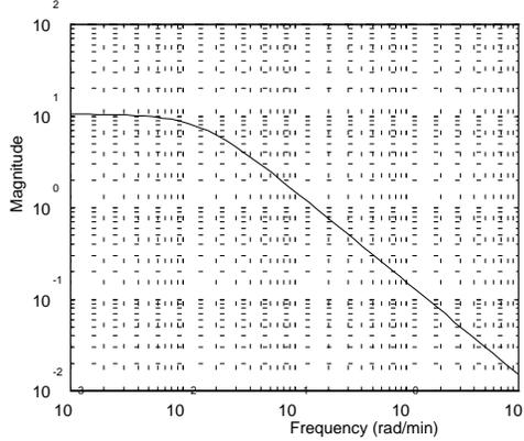
Figure 1. Frequency response of  $G_{ii}(s)$ .
