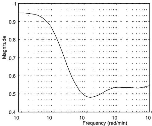
Figure 11. The  $\mu(Q)$  condition for robust performance, Equation 13, (SU).
