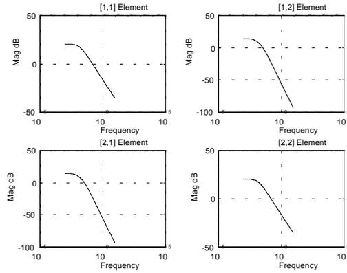
Figure 2. Bode diagrams of the open loop system.
